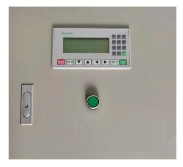
Step 7: The COM, X0, X1, and X2 of control box are respectively connected with the COM,Up, Down and stop of the manual button by a 4-core 1 square line. Test the manual button.
