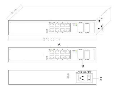
A. PoE Power Port C. 100-240VAC, 50/60Hz B. Combo ports (SFP/RJ45)
