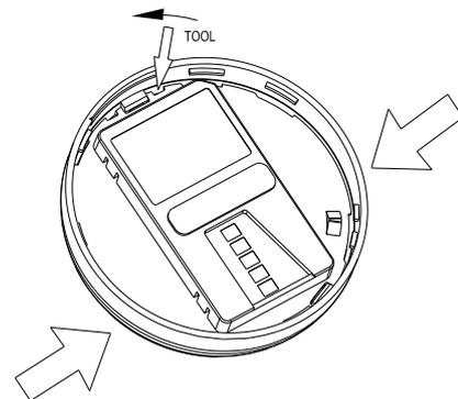
Remove the cover, open the sensor chamber and carefully clean it.
