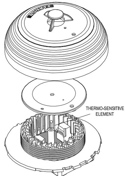
Reassemble the detector, mount it on the connection base and execute the "Immediate Maintenance" as described in the Control Panel's programming manual.
