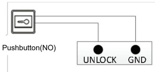
**Note:** This wiring is not polarised.
