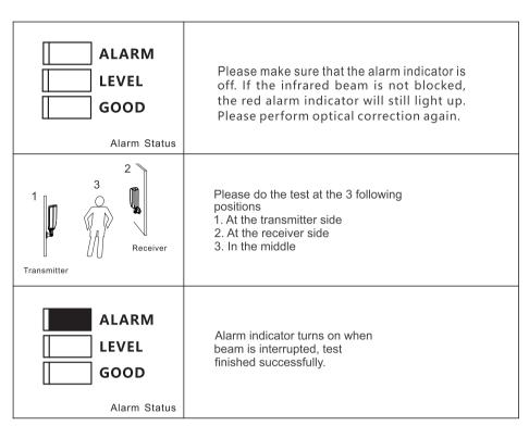
Note: If the alarm LED indicator is OFF even though the beams are completely blocked, refer to the "Trouble Shooting".
