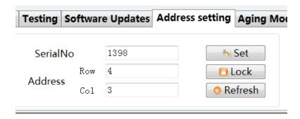
input 1398 in SeralNo., 4 in Row, 3 in Col and click Set button, "Address set successfully" will be displayed on the screen 15, then click the Lock button, the address will be locked.
