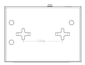
Distance of the mounted holes is 55mm
