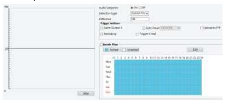
Select Enable for Audio Detection, select a detection type and set the difference or threshold. To disable audio detection, clear the Enable check box.
