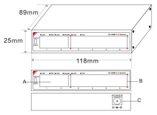
A.2\* Uplink port B. 4\*Gigabit PoE Port C. power DC48V
