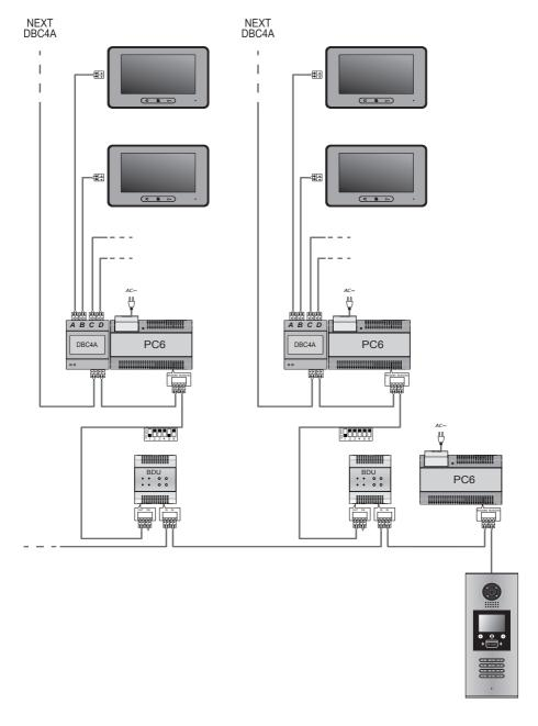
3.3 Gateway Mode: In this mode, the first door station can call all the monitors and can connect up to 8 BDUs, and each BDU can connect up to 32 monitors.
