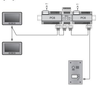
3.2 Router Mode: In this mode, the system can connect up to 8 BDUs, and each BDU can connect up to 32 monitors.
