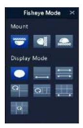
Three mounting modes are available: ceiling, wall, desktop. Ceiling and desktop mounting modes use the same dewarping method.
