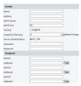
**2.** Configure relevant parameters of the sender and the recipient. Some camera models support Email test. You may test email after setting the recipient address. The following table describes some major parameters.
