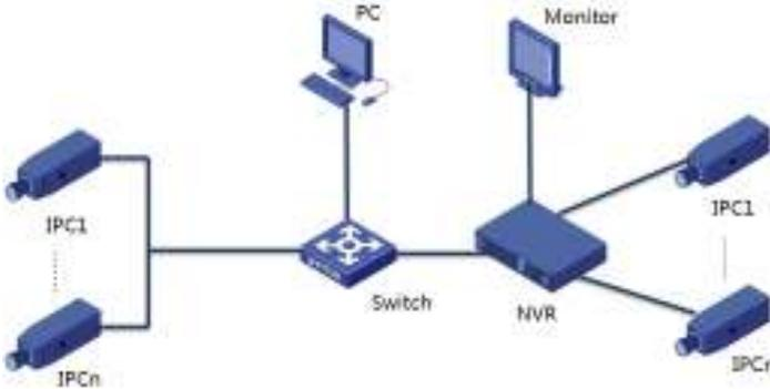
The NVR, IP cameras, and PC are connected on a private network (or LAN). The IP cameras can be connected to the NVR directly or via a switch. And you manage the NVR and the connected IP cameras through the monitor or using a web browser on the PC.
