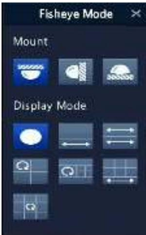
Three mounting modes are available: ceiling, wall, desktop. Ceiling and desktop mounting modes use the same dewarping method.
