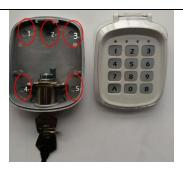
3. Locate the base where needs to install, mark the 5 opened holes in order to fix them.
