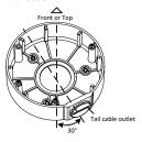
Tail cable outlet of the of the device is drawn junction box.
